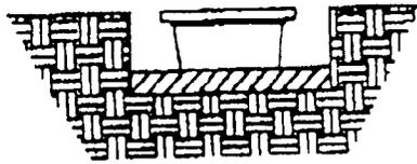
2. Set depth with top edge of the box flush with the finished floor.
