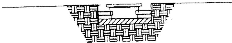
8. After concrete is allowed to set, remove 3/4" plywood to access box. Save the plywood to use when pouring box lid. Do not insert the screws when pouring the lid.
